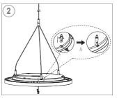
To secure rope onto the fixture, insert the T-shaped rivets to the slot on the reverse of holes on ceiling. Fasten the rope clamper the base, then tighten the rope clampers
