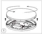
Twist the diffuser anticlockwise. Vertically remove the diffuser and PCBA.
