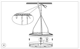
a. Cut off the power. Thread the input cable through the rubber plug to the fixture. Connect the L, N wire referring to the wiring diagram.
