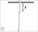
Knock the rawl plugs into the pre-drilled onto the ceiling with screw as shown.
